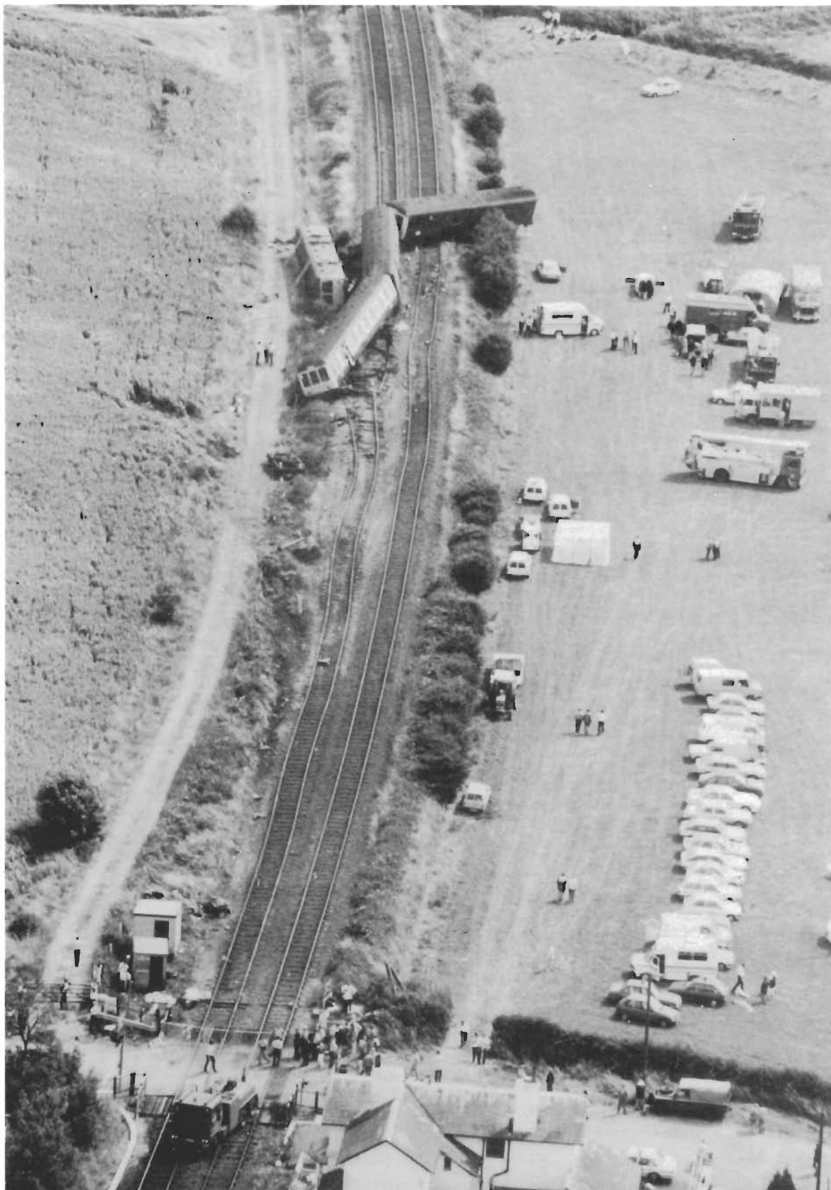
View looking south from crossing. Crossing equipment can be seen at bottom left-hand corner. Leading coach of train is on its side separated from other coaches and facing back towards Bridlington.
